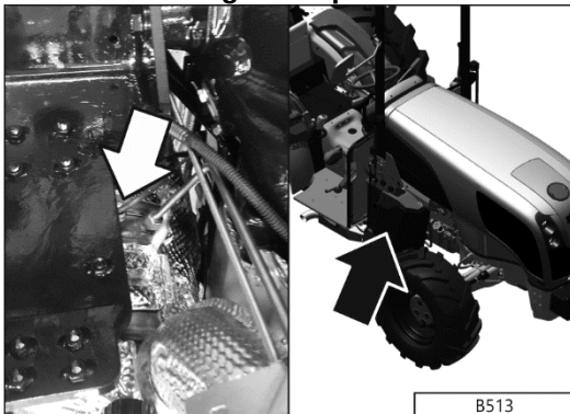
B513 - Exhaust gas temperature sensor 2
